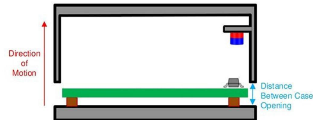
use of a 3D Hall sensor with gain and offset corrections supports flexibility when placing the sensor relative to the magnet, ensuring the most accurate angle calculations.
