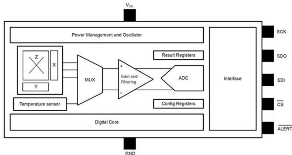
Figure 5: Except for an SPI interface (shown above) on the TMAG5170 models and an I<sup>2</sup>C interface on the TMAG5273 models, the internal functional blocks are the same for both families of 3D Hall effect sensor ICs.
