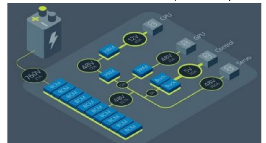
Figure 1: This PDN for 15.4kW agricultural harvesting robots comprises a 760 volt distribution bus supporting a network of lower voltage converters (DCMs, PRMs, NBMs, and buck). *Image source: Vicor*
