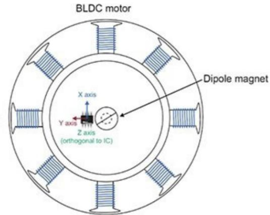
Figure 4: Gimbal motors in handheld camera platforms and drones benefit from 3D Hall effect sensors with selectable magnetic field sensitivity ranges.
