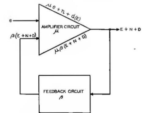
Fig. 1—Amplifier system with feedback.
