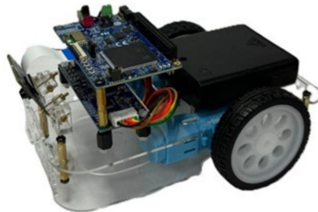
Figure 1: The STEVAL-ROBKIT1 from STMicroelectronics.
