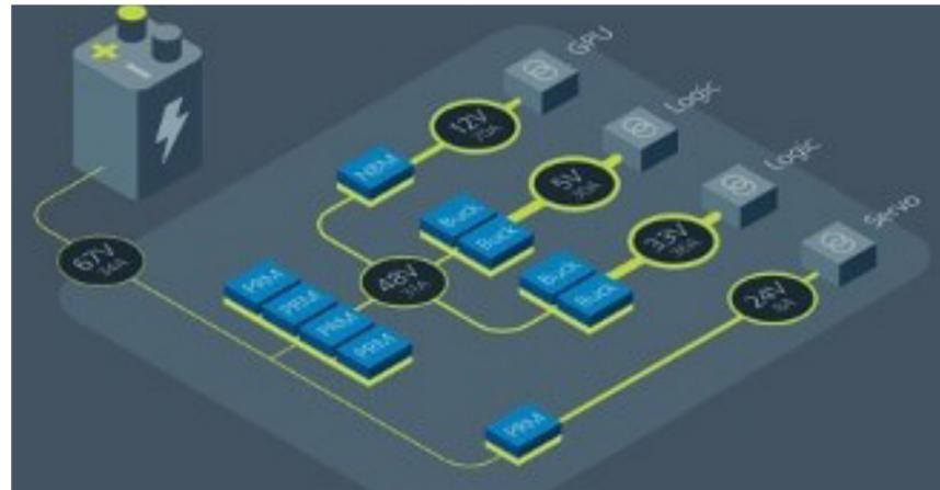
step-down sections that deliver the needed power to the subsystems. A high-voltage power distribution bus results in improved efficiency and lower power distribution currents which allows the use of smaller, lighter and less expensive power cables. The fourth application shows the simplification that can result in smaller robots that use 48 volt battery systems.
