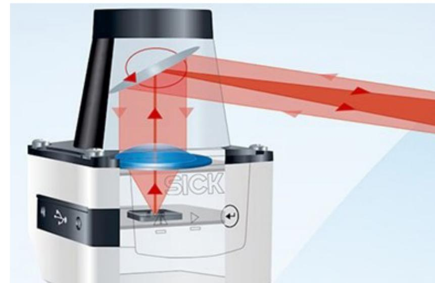
scan their surroundings using optical time-of-flight (ToF) technology. ToF is implemented by sending laser pulses using a rotating mirror and detecting the reflected light. The longer it takes for the reflected light to arrive back at the sensor, the further away the object.
