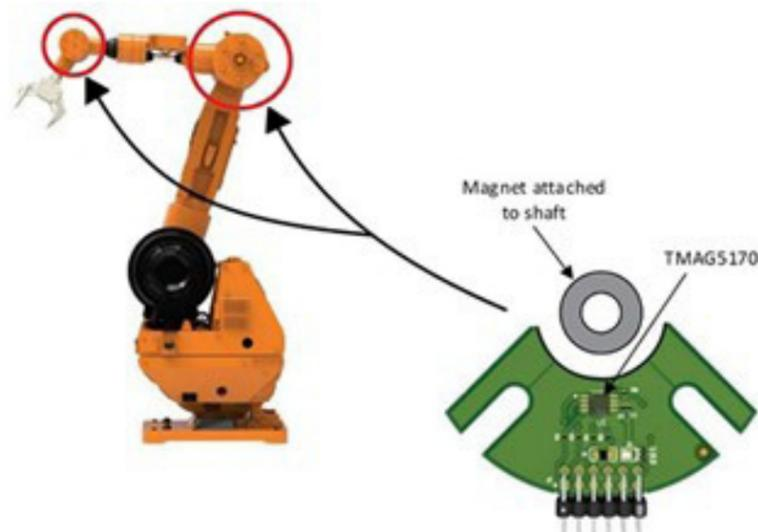
Figure 2: Integrated 3D Hall effect sensors can measure shaft rotation in robots and other Industry 4.0 applications. Image source: Texas Instruments
