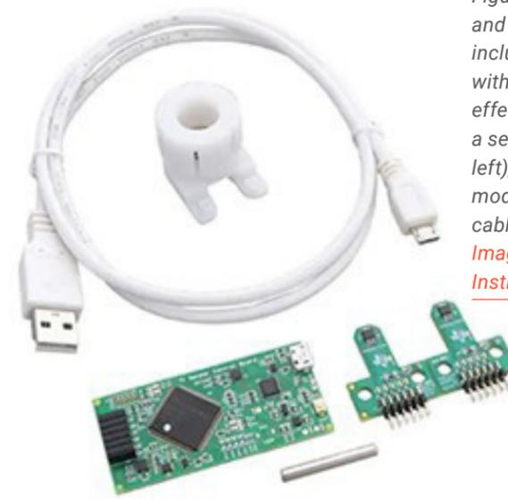
Figure 6: The TMAG5170EVM and the TMAG5273EVM both include a snap-apart board with two different 3D Hall effect sensor ICs (lower right), a sensor control board (lower left), 3D printed rotate and push module (center), and a USB cable to provide power.
