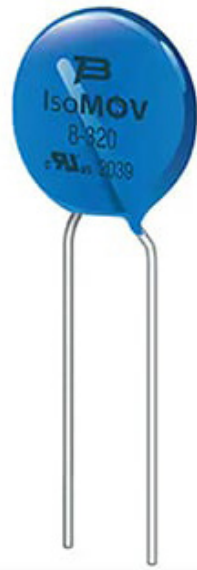
Figure 5: The ISOM3-175-B-L2 is an example of the IsoMOV hybrid protector's compact form factor. Although it includes two MOVs and a GDT, it measures just 13.2 mm in diameter with a thickness of 6.1 mm. (Image source Bourns)
